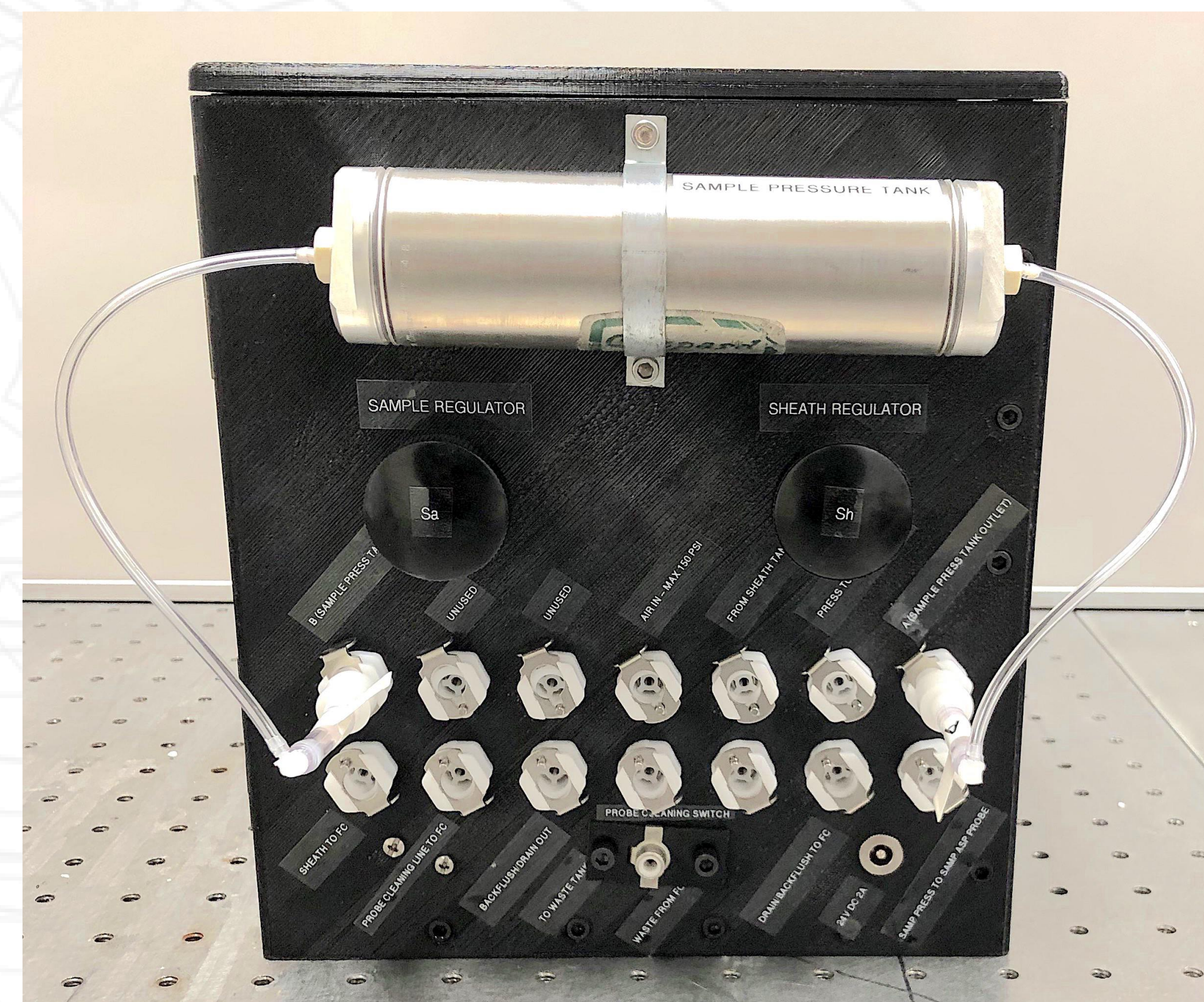
Figure 2. The Shasta Fluidics Control Module uses all analog-controlled valves to regulate flow and quick disconnects for simple hookup.
