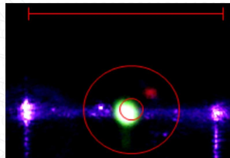
Figure 3. Core stream generated using the Shasta (fluorescein excited with a 405-nm laser). Bar = 404  $\mu\text{m}$ .
